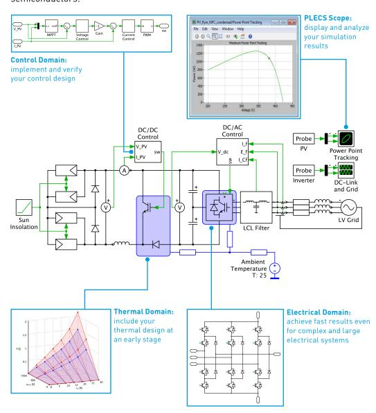
PLECS® is the tool of choice for high-speed simulations of power electronic systems. It is available in two editions: PLECS Blockset for seamless integration with MATLAB®/Simulink®, and PLECS Standalone, a completely independent product.
