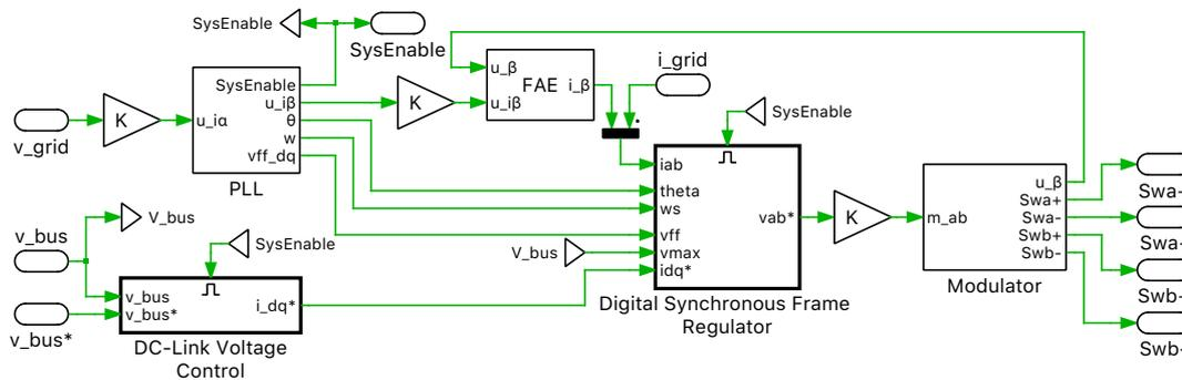
**Figure 4: Inverter controller**
