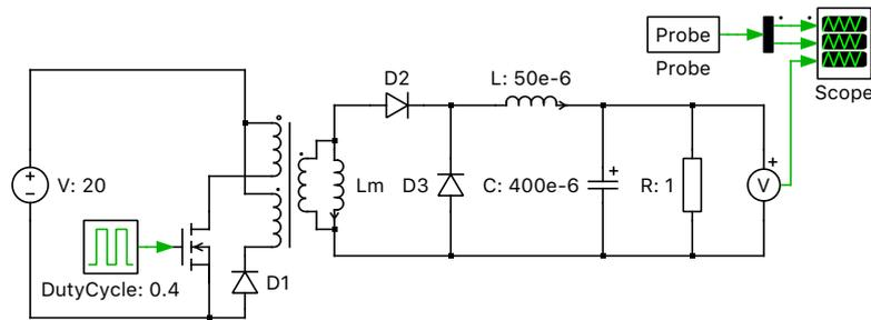
**Figure 1: Forward converter**
